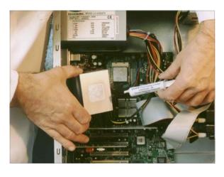
contact area available. Generally it is necessary to use a suitable interfacing material to compensate for surface discrepancies of roughness and undulation. Wherever possible, close fitting, solder brazed interfaces provide the most satisfactory solution.
